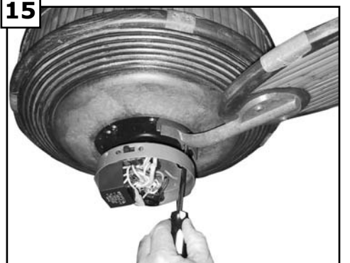
15 Check the motor for plastic shipping stabilizer tabs, and remove them if they are present. The screws, washers and motor pads are pre-installed to the blade holders. Attach blade assembly to motor and tighten screws securely.
